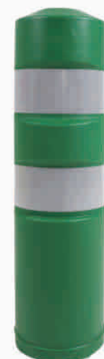
Item No.:GMP-E05 (Flex Bollard) Material : PE (polyethylene)--rugged and durable, Top & Base elastic joint ensures bollard returns to upright position, Molded rings accept a range of ropes or chain
